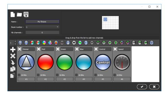
You can easily create a new fixture profile using drag from the list of common channel icons and drop from into the area under the list.
